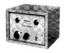
Resisteral Temperature Controller manufactured by Hallikainen Instruments designed for installations where precision temperature control is required. The instrument uses a resistance type temperature bulb, suitable for temperatures up to  $600^{\circ}$ F. Various types of bulbs are available, for installation in pressure vessels, baths, and ovens PF6
